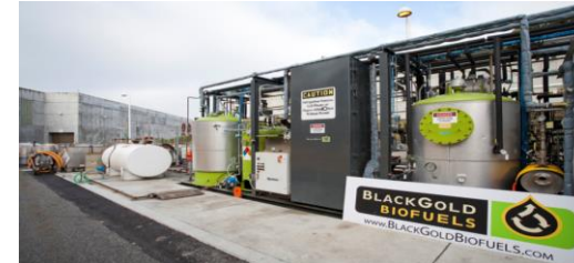
Biodiesel Production System (bottom) at San Francisco's Oceanside Wastewater Treatment Plant (Source: SFPUC)
