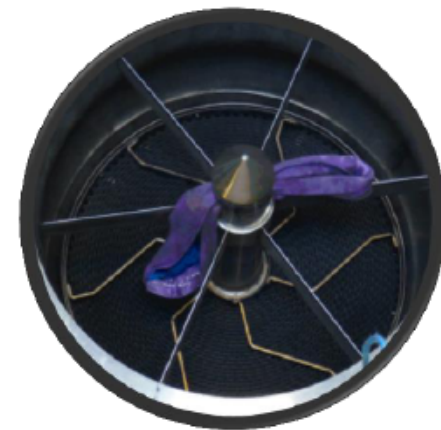
Figure 3: Monolithic tar reformer catalyst
